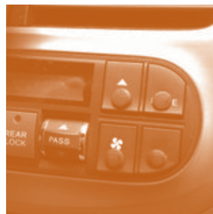
Figure 3: Sugru shaped into round flat buttons added to control panel in van to make functions easier to activate.
